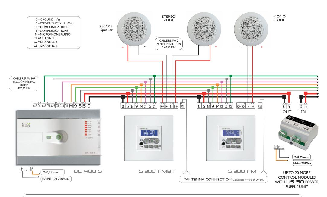
NOTE: The UC-400S central unit supports a maximum of 10 control modules and a máximum distance to the last element to control of 100 meters of cable. For higher installations, the installation of extra power supply units or a more powerful central unit is a must. \*In zones of bad reception, connection to outdoor antenna it is highly recommended.
