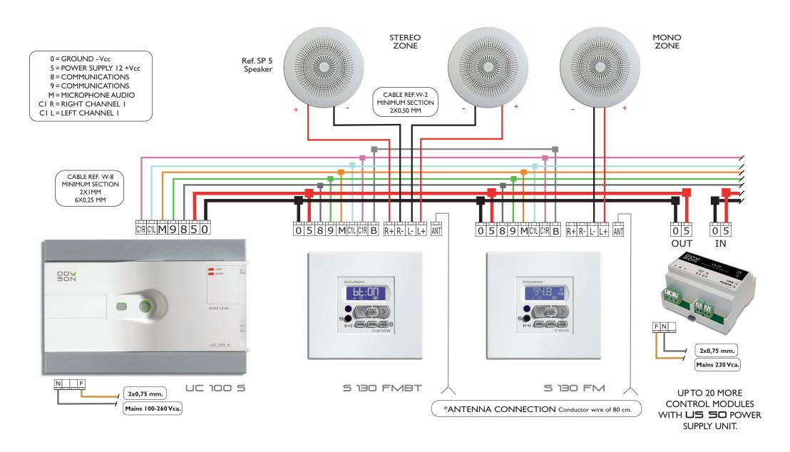
NOTE: The UC-100S central unit supports a maximum of ten control modules and a maximum distance to the last element to control of 200 meters of cable. For higher installations, the installation of extra power supply units or a more powerful central unit is a must. \*In zones of bad reception, connection to outdoor antenna it is highly recommended.
