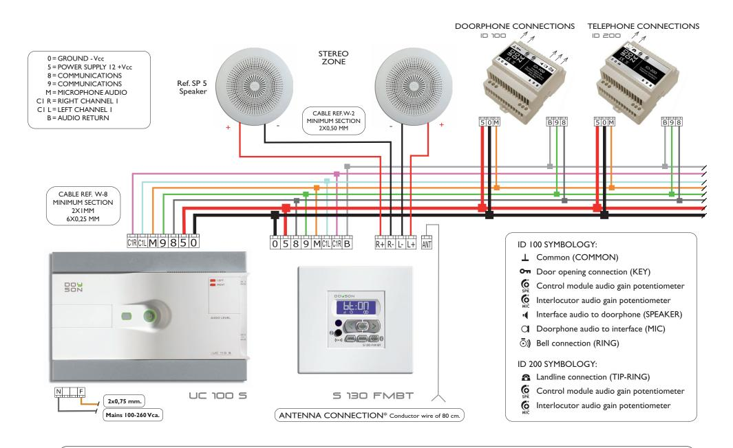
Note: "B" only must be connected when ID100 and ID200 interfaces are present on the sytem. \*In zones of bad reception, connection to outdoor antenna it is highly recommended.
