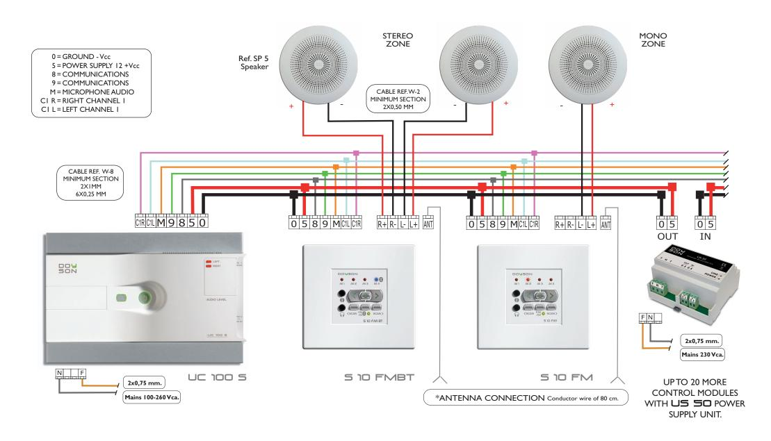
NOTE: The UC-100S central unit supports a maximum of ten control modules and a máximum distance to the last element to control of 200 meters of cable. For higher installations, the installation of extra power supply units or a more powerful central unit is a must. \*In zones of bad reception, connection to outdoor antenna it is highly recommended.
