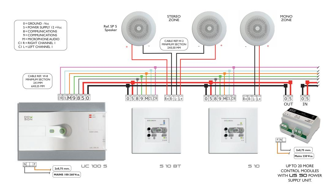
NOTE: The UC-100S central unit supports a maximum of ten control modules and a máximum distance to the last element to control of 200 meters of cable. For higher installations, the installation of extra power supply units or a more powerful central unit is a must.
