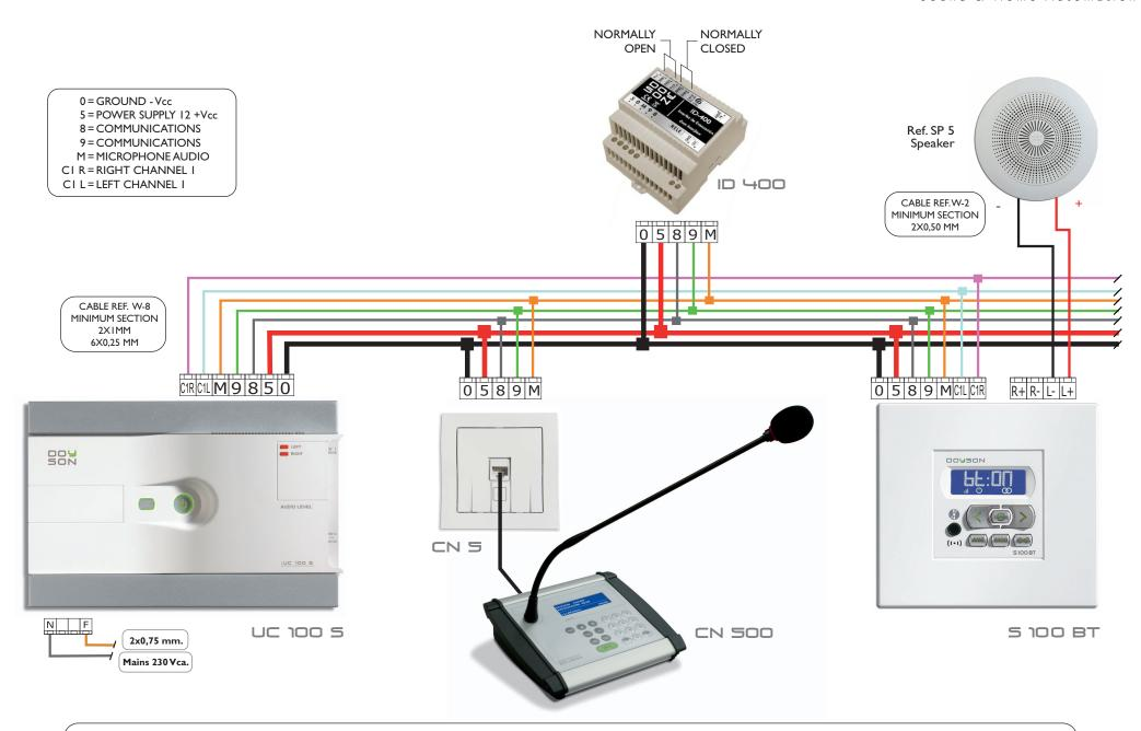
Observations: The CN 500 microphone desk has 2 strips for connecting auxiliary equipment AUX1 and AUX2 and an audio output to attack auxiliary equipment with preference for announcements.
