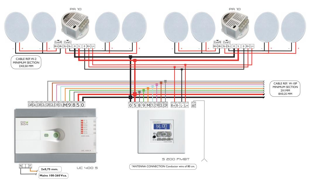
NOTE: The UC-400S central unit supports a maximum of ten control modules and a máximum distance to the last element to control of 100 meters of cable. For higher installations, the installation of extra power supply units or a more powerful central unit is a must. \*In zones of bad reception, connection to outdoor antenna it is highly recommended.
