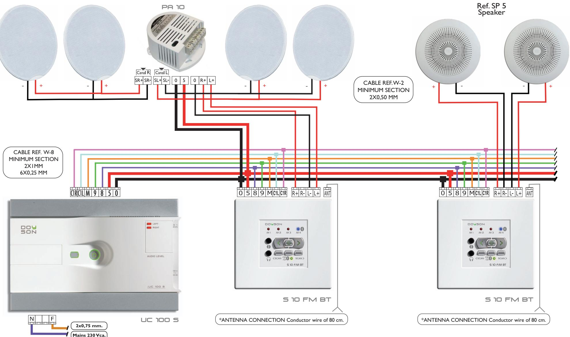
NOTE: The UC-100S central unit supports a maximum of ten control modules and a maximum distance to the last element to control of 200 meters of cable. For higher installations, the installation of extra power supply units or a more powerful central unit is a must. \*In zones of bad reception, connection to outdoor antenna it is highly recommended.
