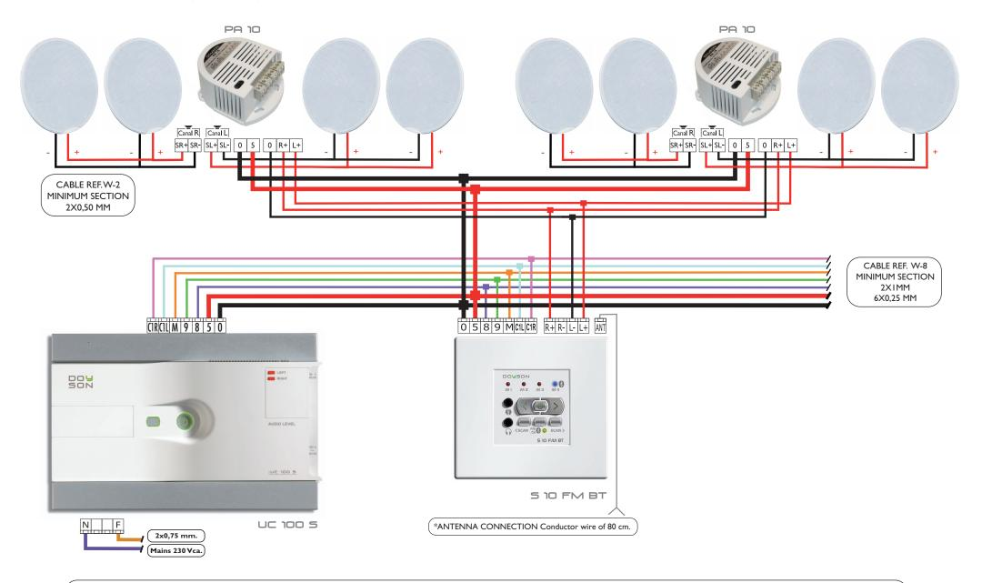
NOTE: The UC-100S central unit supports a maximum of ten control modules and a máximum distance to the last element to control of 200 meters of cable. For higher installations, the installation of extra power supply units or a more powerful central unit is a must. \*In zones of bad reception, connection to outdoor antenna it is highly recommended.
