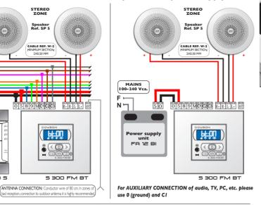
NOTE.- The UC 400 S supports a máximum of 10 sound control modules and a maximum distance of 100 mts.of cable to the last element to be controlled. For higher installations, power supply units or a more powerful central unit would be required.
