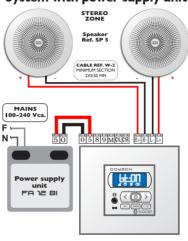
For AUXILIARY CONNECTION of audio, TV, PC, etc. please use 0 (ground) and CIL and CIR (Left and right channel I)
