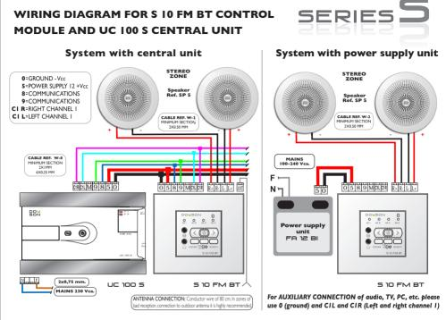
NOTE.- The UC IC Supports a máximum of 10 sound control modules and a maximum distance of 100 mts.of cable to the last element to be controlled. For higher installations, power supply units or a more powerful central unit would be required.
