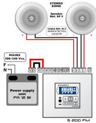
For AUXILIARY CONNECTION of audio, TV, PC, etc. please use 0 (ground) and CIL and CIR (Left and right channel 1)
